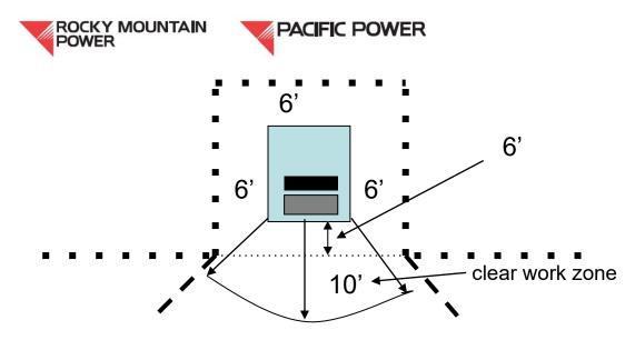
Figure 2 – Clearance Around a Metallic Fenced Enclosure
