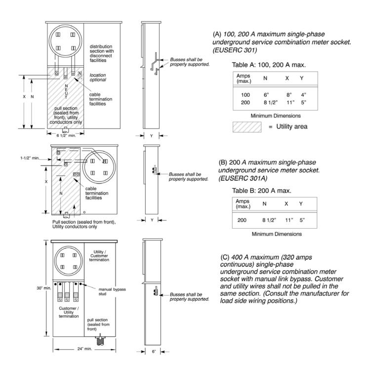
Figure 21—Residential Underground Approved Meter Sockets
