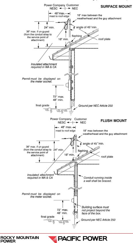
Figure 8—Overhead Service to Wall-Mounted Meters
