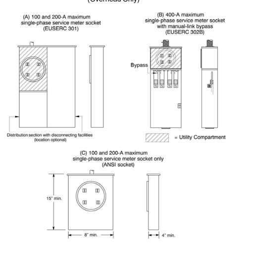
Figure 20—Residential Overhead Approved Meter Sockets (Overhead Only)
