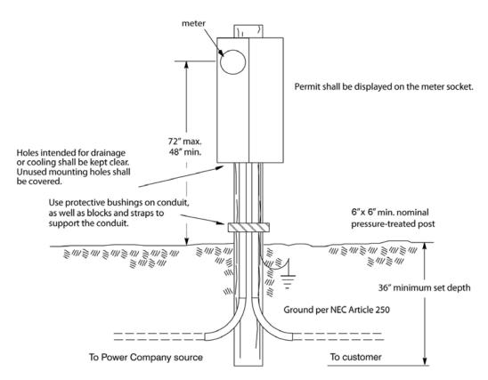
Figure 28—Underground Service to a Free-Standing Meter Socket, Manufactured Package
