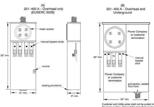
Customer and Utility wires shall not be pulled in the same section. (Consult the manufacturer for load side wiring positions.)
