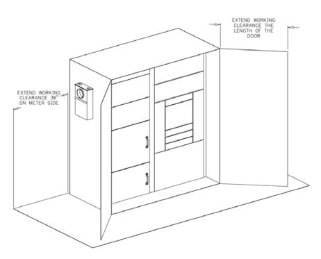
Figure 37—Flat Surface Around a Switchboard Enclosure
