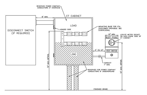
Figure 51—Typical Installation of 800 A CT Metering Installation
