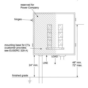
Figure 37—Example of Workspace in CT Cabinet with Bottom-Entry Line and Load
