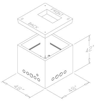
Figure 50—A Typical Vault for a Single-Phase Pad-Mounted Transformer (SI# 7999607)
