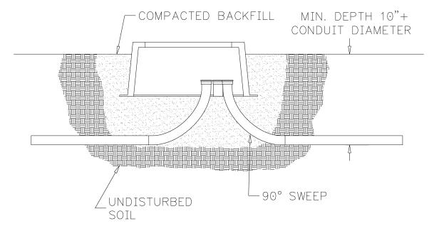
Figure 63—Side View of Secondary Box with Flat Lid
