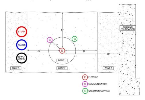
Figure 9—Minimum Separation of Paralleling Lines and Structures
