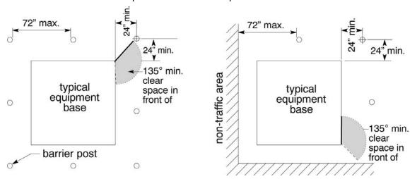
Figure 44-Barrier Post Layout and Clearances
