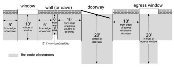
Figure 42—Clearances Between Equipment and Structures
