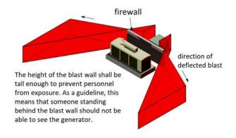
Figure 43—Typical Firewall
