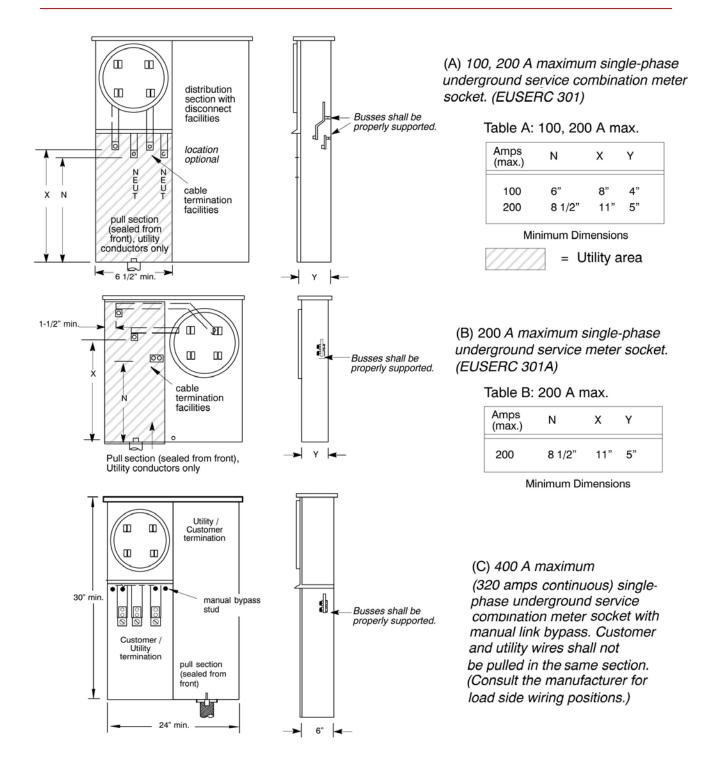
Figure 34—Residential Underground Approved Meter Sockets
