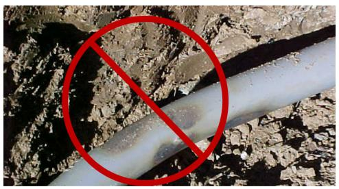
Figure 17—Field-Altered Sweep - Damaged PVC
