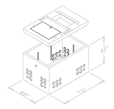
Figure 54—A Typical Vault for a Single-Phase Sectionalizing Cabinet (SI# 7992975)
