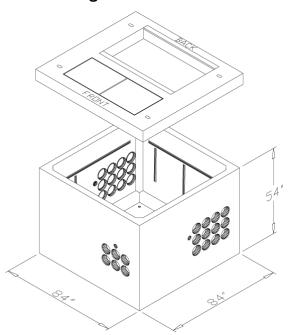
Figure 55—A Typical Vault for a Type 3 Switchgear (SI# 7992787)
