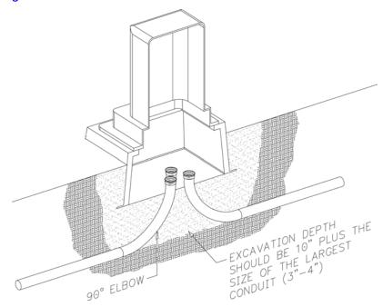
Figure 62—Isometric View of Secondary Box with Pedestal
