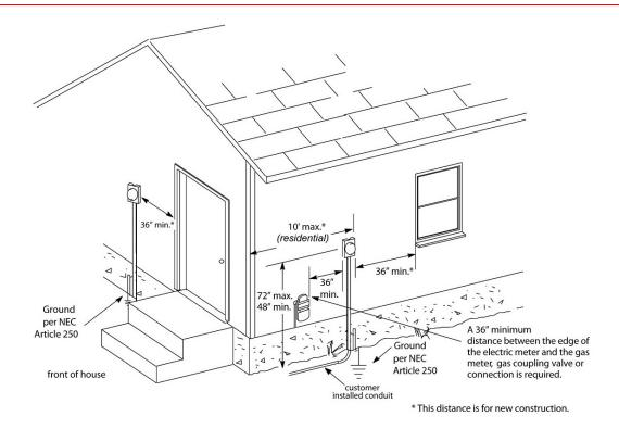
Meter Attached to Dwelling (UG) The customer provides the trench, conduit and sweeps. All above-ground 10' max. conduit shall be Schedule 40 or better. 72" max. 36" min 48" min. WEW SWEW 24" min. customer installed conduit Minimum 36" sweep 2 Customer maintains conduit in and on structures, Coupling of sweep shall including sweeps and swedges. be outside of footing The Power Company owns conductors to the conductor landing in the customer meter socket.
