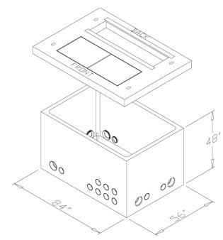
Figure 53—A Typical Vault for a 15 kV Three-Phase Sectionalizing Cabinet (SI# 7992605)
