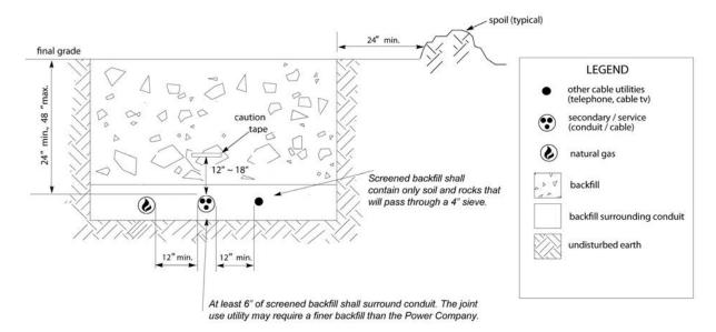
Figure I I—Joint Use Primary Trench
