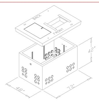
Figure 5 I—A Typical Vault for a Single-Phase, Pad-Mounted Transformer with Opening (SI# 7992977)
