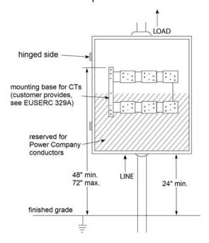
Figure 35—Example of Workspace in CT Cabinet with Top-Half Load
