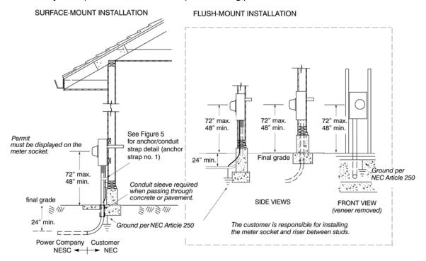
Figure 33—Underground Service to Wall-Mounted Meters
