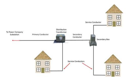
Figure I—Primary, Secondary, and Service Conductor Schematic
