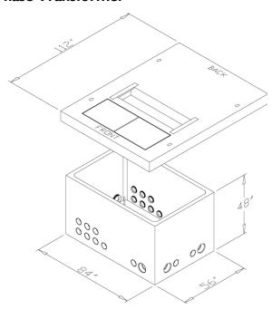
Figure 52—A Typical Vault for a 75-750 kVA Three-Phase Pad-Mounted Transformer (SI# 7992600)
